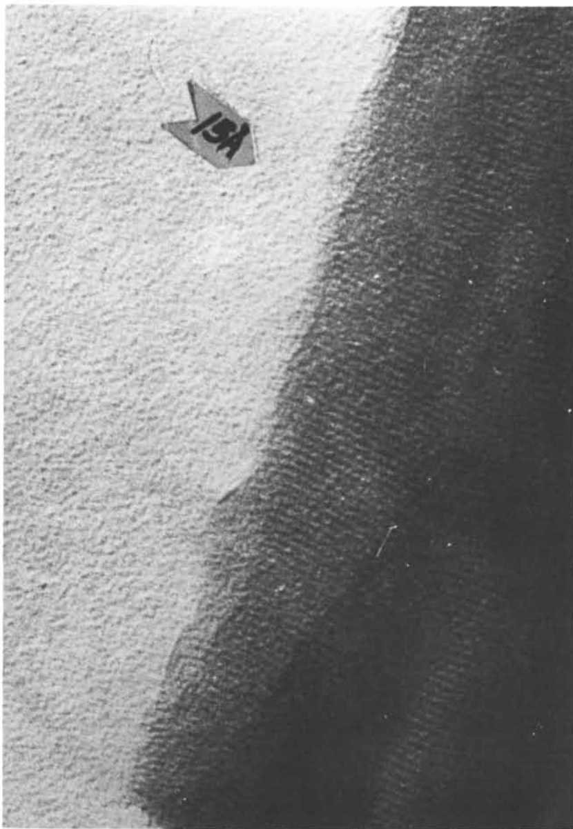
Figure 10. Transmission electron micrograph of the compound Zr(O_3PC_6H_{13})_2 , at 540,000 power. The layer-layer stacking is apparent in profile, with a repeat distance of about 15Å.
